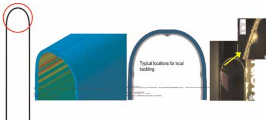
Figure 15. Predicted local buckling on a film stack bonded with an OCA with a stiffness of 10% of that of 3M™ CEF35. The inserts are the photos of a local buckling on the actual film stack.
