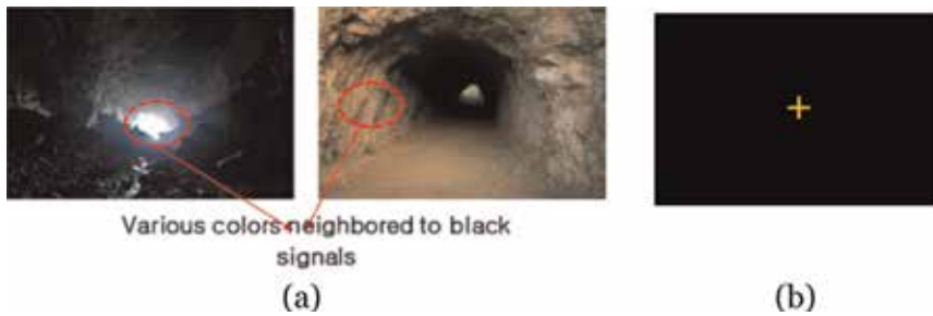
Figure 4. Example of various colours around black signals in complex images and conventional black test pattern. (a) Black signals in complex images and (b) full-screen black [6].
