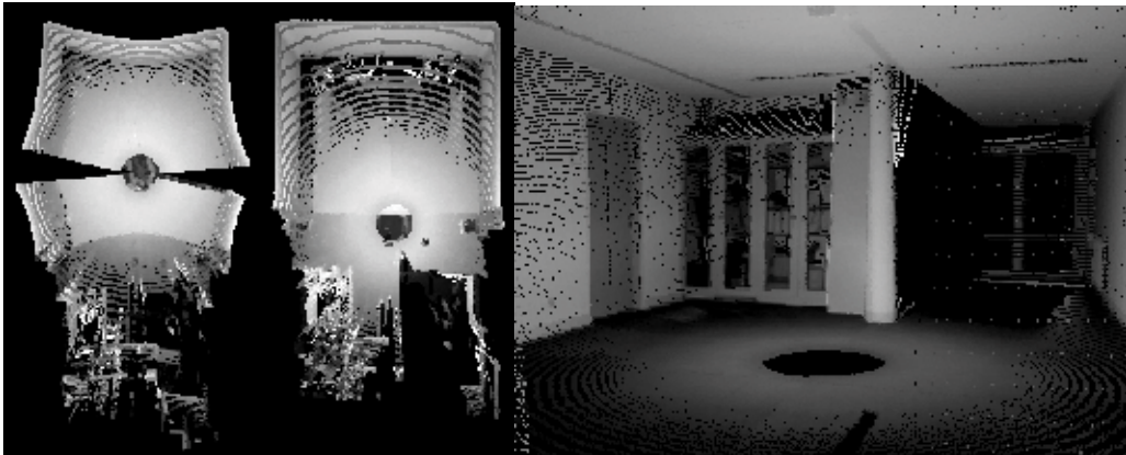
Fig. 3. a) Scan results without and with pose correction. b) 3D scan with remission values.
