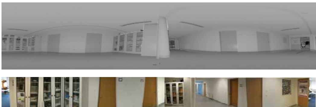
Fig. 4. Top: Panorama view generated with the remission values of the 3D scan. Bottom: Panorama generated by second turn of the robot with the panorama software hugin. 11
