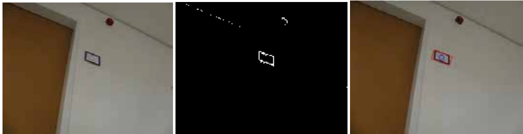
Fig. 10. Example of the filtering process. Left original image, middle binaries image and right annotated doorplate.
