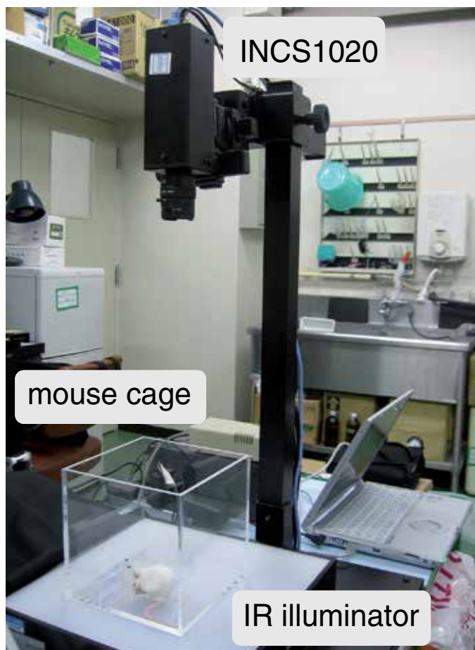
Fig. 4. An overview of real-time scratching quantification system.
