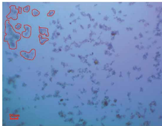
Figure 8. Floc number manually counted from the microscope images. The red part showing the individual floc can be recognized manually for further statistical analysis.
