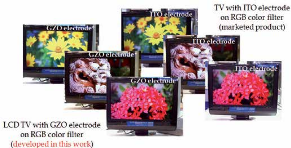
Fig. 14. Comparison of the display pictures between 20 inch LCD TVs with GZO and ITO electrodes on the RGB color filter.
