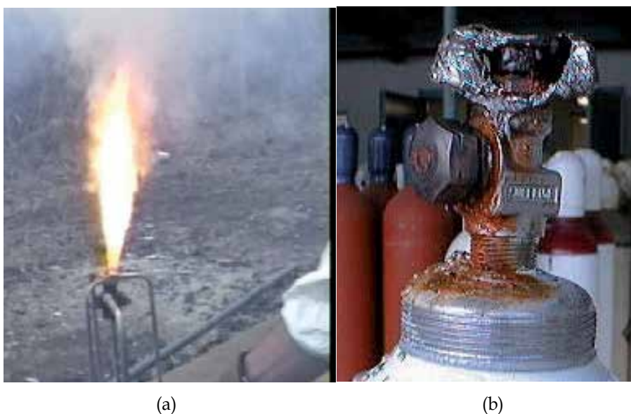
Fig. 3. Typical phosphine combustion flame and powder. (a) Orange flame and white phosphorous pentoxide powder (b) Red phosphorus powder.
