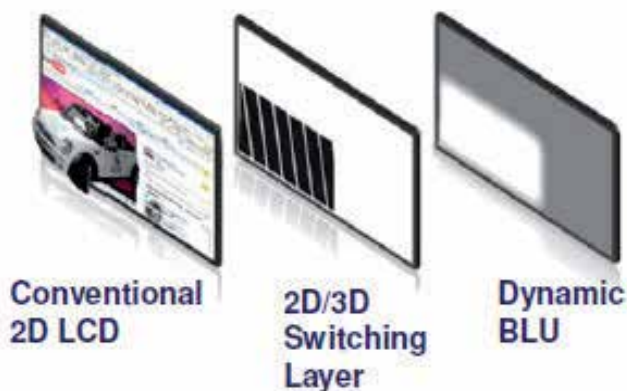
Fig. 13. The structure of 2D/3D switching design for integrated 2D/3D display
