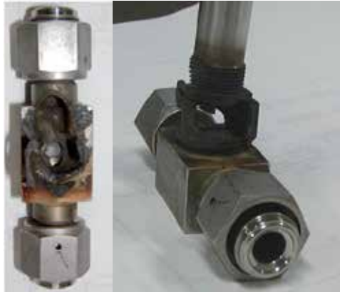
Fig. 5. A burnt valve in a nitrogen trifluoride line caused by adiabatic compression.
