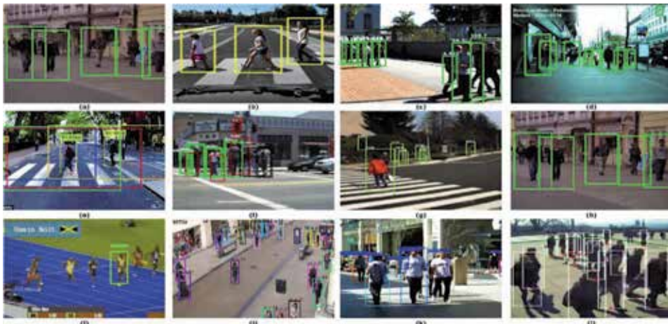
Figure 5. Example of pedestrians detection and tracking. (a) Detecting pedestrians outdoors, walking along the street. (b) ADAS pedestrian detection. (c) Pedestrian detector is based on the aggregate channel feature detector. (d) Real-time vehicle and pedestrian detection of road scenes. (e) Pedestrian action prediction is based on the analysis of human postures in context of traffic. (f) Pedestrian detection based on hierarchical co-occurrence model (g) Cross-modal deep representations for robust pedestrian detection. (h) Pedestrian detection OpenCV. (i) Object tracking with dlib C++ library. (j) Multiple object tracking with Kalman tracker. (k) Multi-Class Multi-Object Tracking using Changing Point Detection. (l) Pedestrian tracking using Deep-Occlusion Reasoning method.
