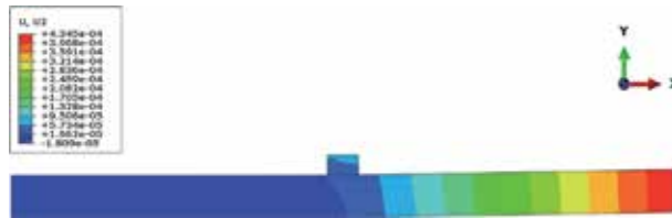
Figure 13. Deflection of substrate along y (m).
