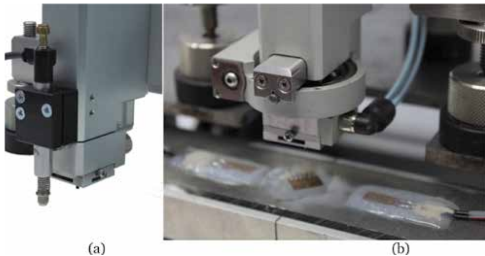
Figure 1. (a) LVDT sensor installed on the drilling device and (b) orbital drilling slide.
