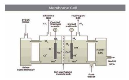
Figure 4. Electrolysis chamber (electrolizer and cell membrane).
