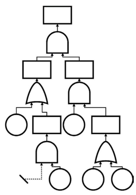
**Figure 6.** *Fault tree example. Own elaboration.*
