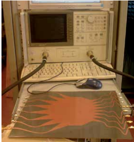
Fig. 6. Fabricated 8×8 ITS Rotman Lens Microwave BFN.
