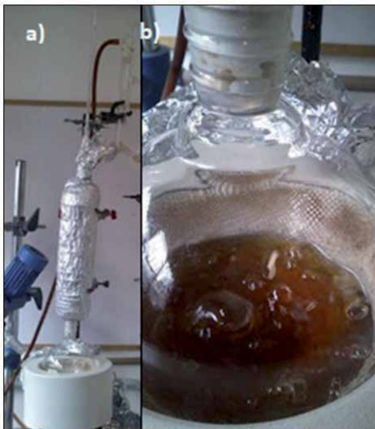
Figure 5. (a) Fractional distillation equipment and (b) reaction mixture to be distilled.
