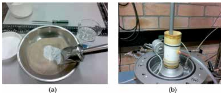
Figure 15. Procedure of (a) mixing and (b) molding bio-cemented samples for triaxial test.
