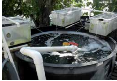
Figure 7. A circular holding biofilm tank without plastic liner, and three aquaria with plastic sheer liner above, used for the second and following holdings.
