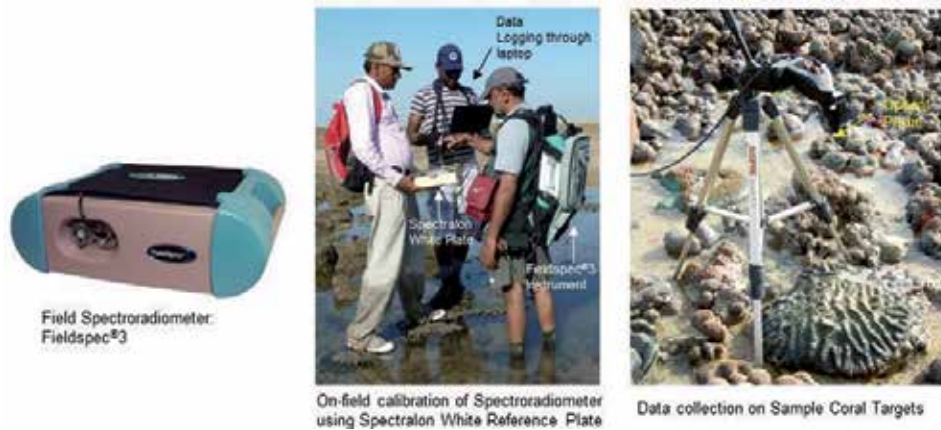
Figure 2. Field spectroradiometer and in situ hyperspectral data collection at Laku Point reef site, India [5].
