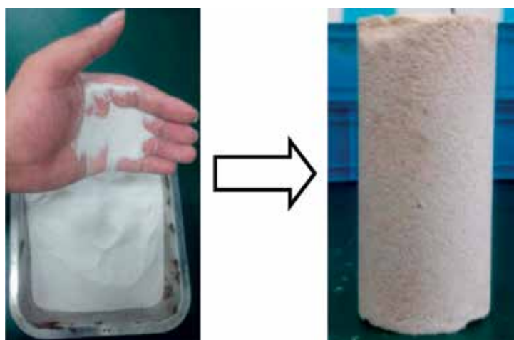
Figure 11. Loose sand particles to sand column cemented by biocomposite cement.
