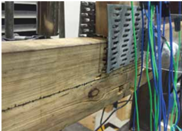
Figure 8. The lower chord cracks accompanied by tooth extraction test process of SPT-S1.
