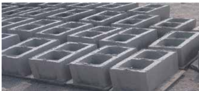
Figure 2. Freshly manufactured concrete hollow blocks.
