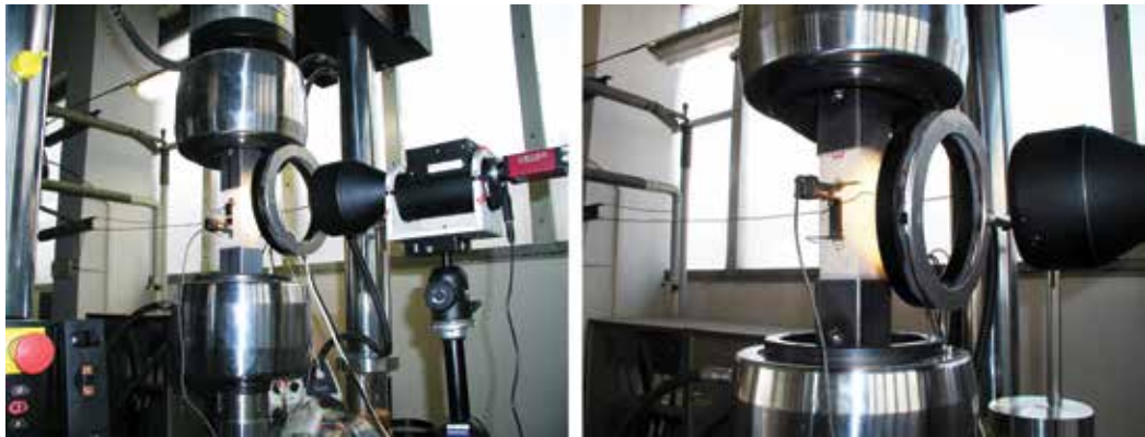
Figure 5. Arrangement of pure tension tests on the stone specimens (photo by M. Šperl).
