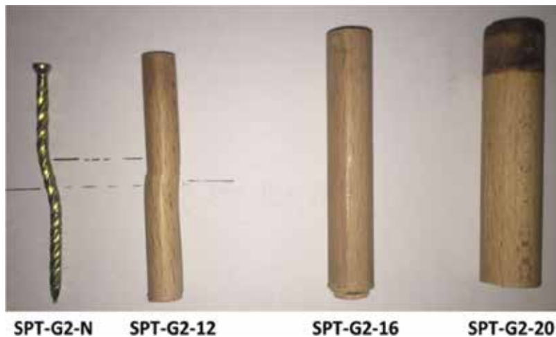
Figure 12. Failure form of connectors.
