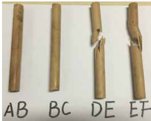
Figure 19. Failure of connectors in SPT-G3-16.
