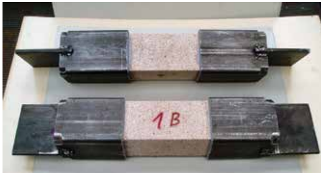
Figure 4. Test compression/tension specimens (photo by M. Šperl).
