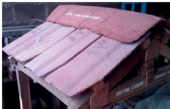
Figure 5. A prototype roof fabricated from rattan-cement composite tiles. Source: [16].
