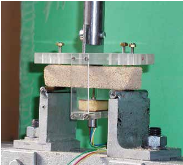
Figure 15. Three-point bending test arrangement (photo O. Vála).
