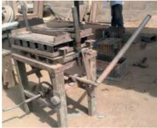
Figure 13. Side view of the tile-making machine. Source: [41].
