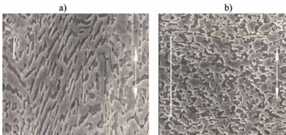
Figure 4. An alloy microstructure after deformation at 920°C and speeds of deformation 1,1 \cdot 10^{-3} \text{ s}^{-1} . (a) \delta = 55\% , (b) \delta = 200\% . \times 1000 .
