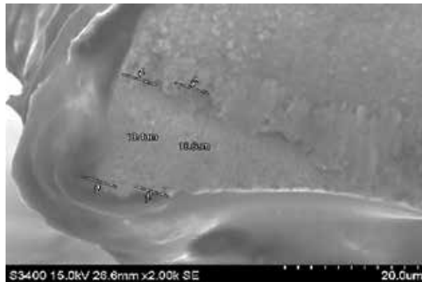
Figure 11. Coated AlTiN tool wear at 70,000 rpm.
