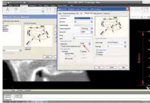
Fig. 31. To adjust Scale factor till the vertical linear dimension value changes identical to the reference ruler value the dimensions created can be observed clearly.
