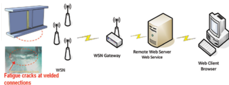
Figure 1. Remote wireless bridge monitoring system.
