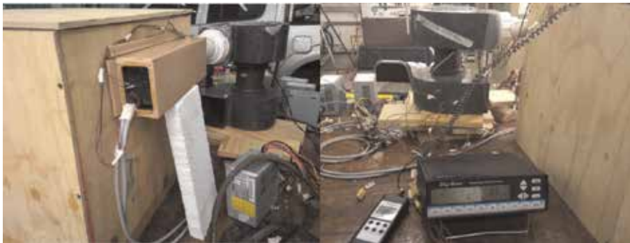
Figure 12. Thermoelectric air conditioner placed inside of testing enclosure.
