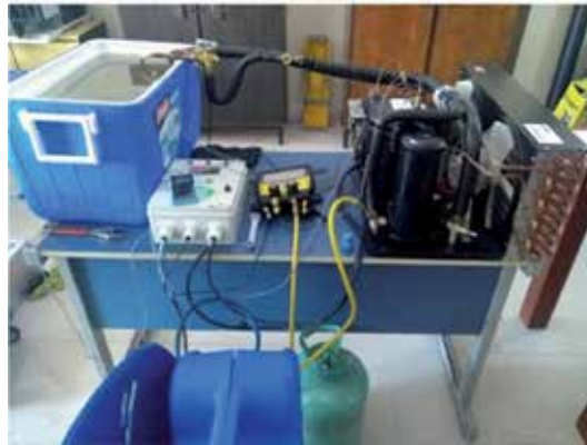
Figure 1. Bench tests with chiller mounted by ClimaTConT.
