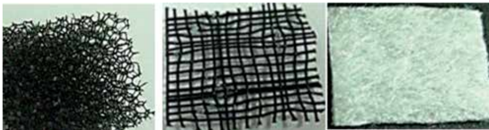
Figure 11. Structure of filters observed under an optical compound microscope. The right-hand panel shows sponge filter cavities of different sizes. These openings are wider than those of other filters. The middle panel shows a polyester filter, which is characterized as a network installation with narrower openings than the sponge filter that are regular in shape. The left-hand panel shows a HEPA filter, characterized by complex knit and numerous narrow openings that increase efficiency by preventing the passage of fine particles.
