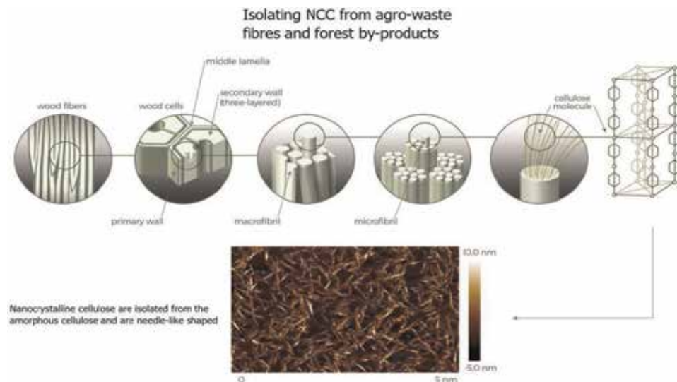
Figure 4. Schematic representation of lignocellulosic agro-waste and by-product of forest classification. Adapted from Ref. [47].
