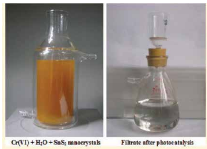
Figure 20. Photodegradation of Cr(VI) in the presence of SnS 2 . Reproduced with permission from [23].
