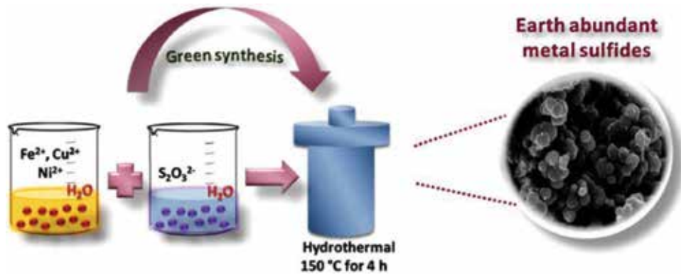
Figure 1. Schematic illustration of the hydrothermal synthesis of \text{FeS}_2 , \text{CuS} , and \text{NiS}_2 powders. Reproduced with permission from [10].
