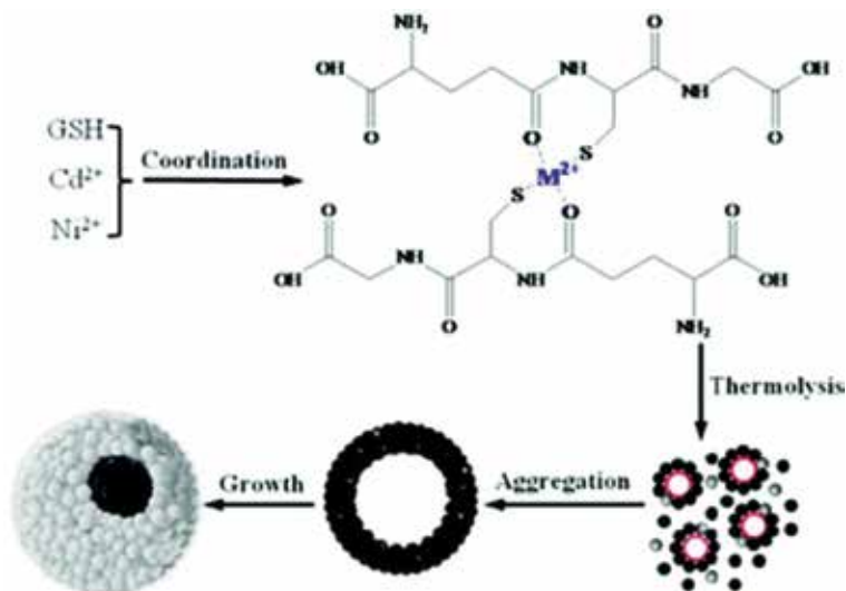
Figure 3. Mechanism for the formation of Ni-doped CdS. Reproduced with permission from [7].
