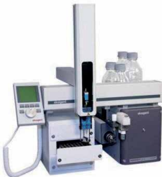
Figure 11. Pictorial representation of LC–MS/MS system with higher loading capacity of autosampler.
