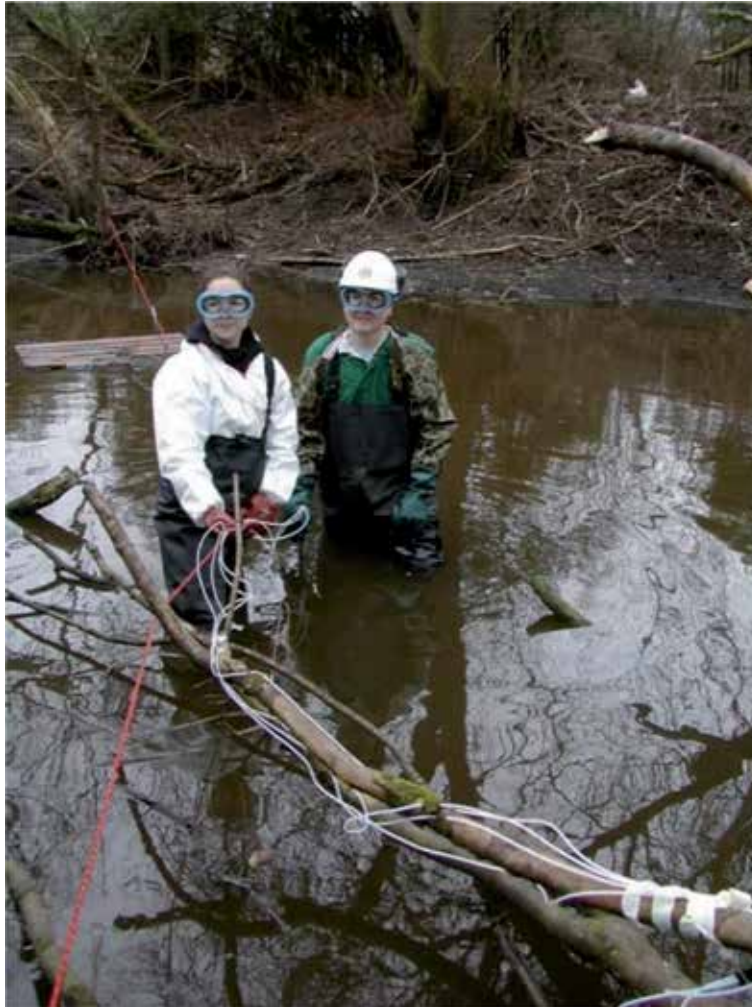
Figure 2. Hyporheic zone multilevel sampling of the bed of Polmadie Burn, Glasgow. Note how, for ease of access, the multipoint sampling tubes were extended from the sampling point to the base station where the peristaltic pump was deployed.
