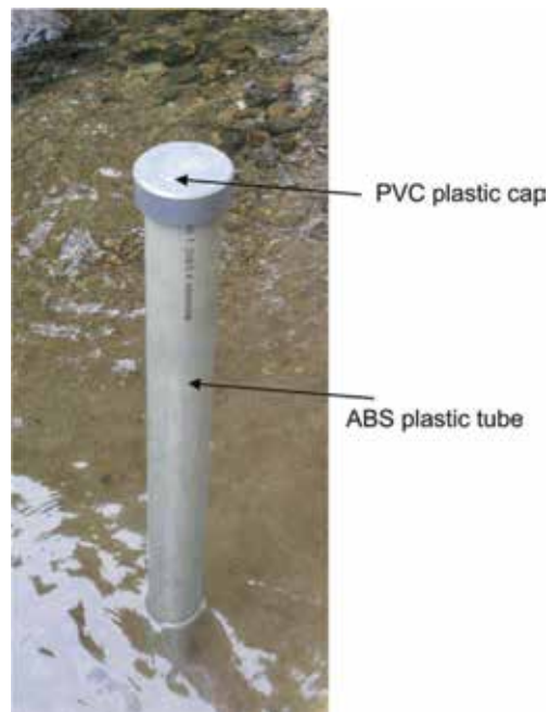
Figure 1. DGT placed in the base of the hollow sampler and left for 24 hours.
