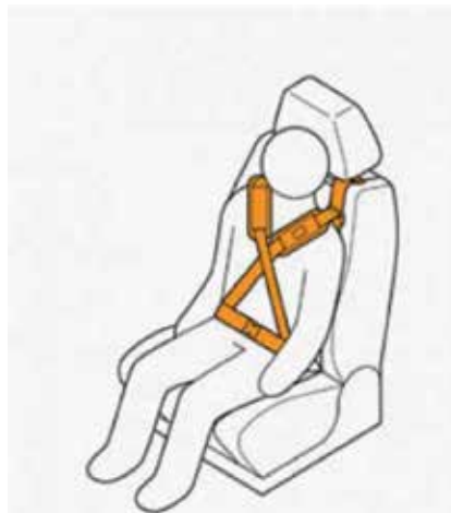
Figure 5. The principle of the Careva Crossit positioning belt [16].
