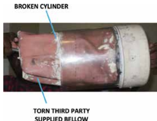
Figure 7. Example of failure during the project.
