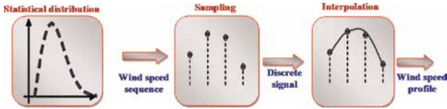
Figure 3. Wind speed generation process.
