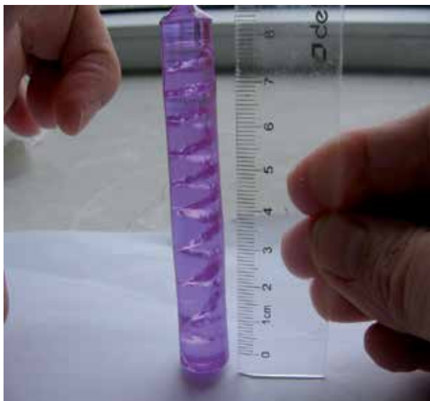
Fig. 2.1 The cracking \text{Nd}^{3+}:\text{NaY}(\text{WO}_4)_2 crystal.
