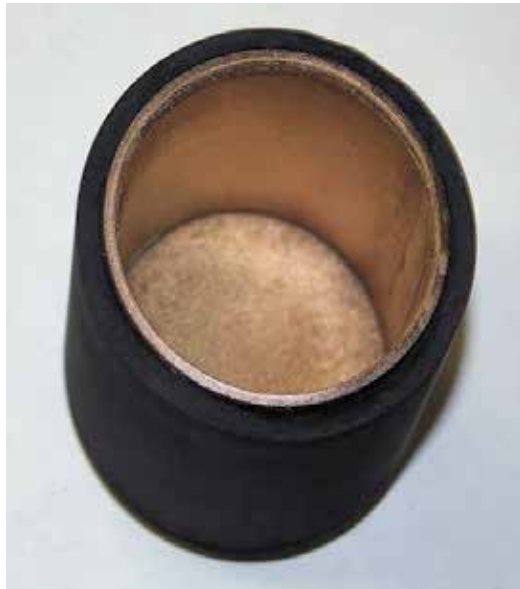
Fig. 9. Ta (dark gray) crucible (diameter 63 mm) completely covered with a layer of TaC-Ta 2 C ceramics (gold) that is converted into TaCN during the growth to prevent the formation of easily melted eutectics (Ta-Si and Ta-Al) (Vodakov et al., 2003).
