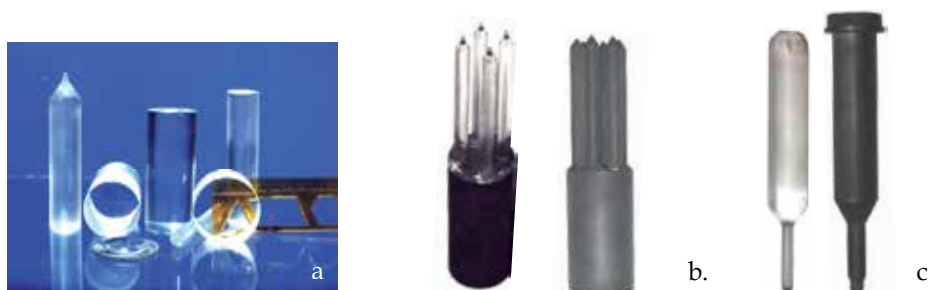
Fig. 2. (a) Calcium fluoride crystals; (b) multiple type crucible; (c) crucible with seed.
