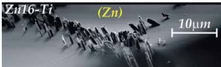
Fig. 10. A strengthening stripe ((Zn) + Zn_{16}Ti ) within the (Zn) – single crystal frozen during its growth in the Bridgman system; the Zn_{16}Ti – rods are all of the same size, mainly.
