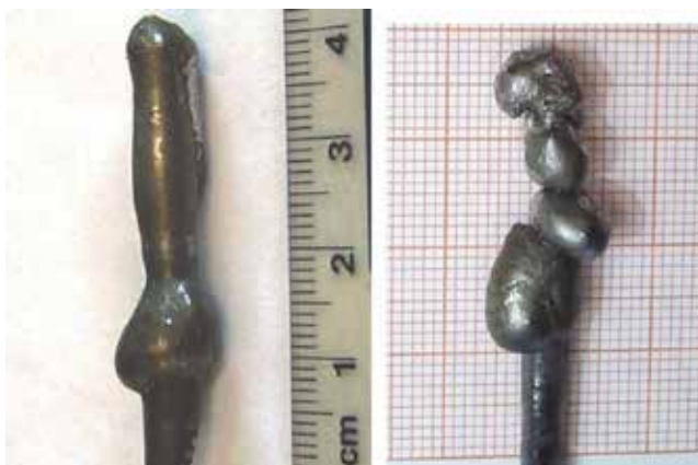
Fig. 2. Samples resulting from crystal growth experiments from the stoichiometric melt with upper and lower rod rotation. Left - Successfully grown single crystal ( sc1 ); Right - The crystallized ingot experienced repeated dropping down of the melt because of the unfavorable combination of the high density and of the low surface tension of the melt.
