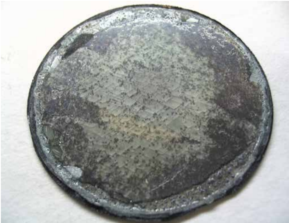
Fig. 11. 2-in AlN seed grown on 60 mm micropipe-free SiC substrate.
