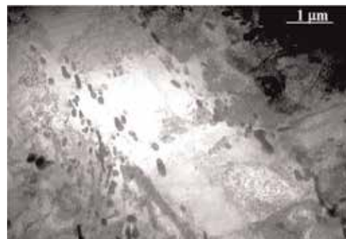
Figure 39. Large ferrite lath in as-welded FB2 HAZ at location near to A1 temperature.
