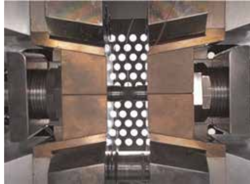
Figure 30. The HAZ-simulated sample in Gleeble chamber during the ACT, before cracking.
