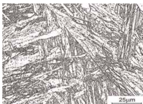
Figure 13. High-tempered martensite of forged 9Cr-1.5Mo-1.3Co-V-Nb-N-B (FB2) steel in as-delivered state, FeCl 3 etched.
