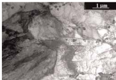
Figure 26. Martensite grain and recrystallized ferrite, in simulated HAZ region close to peak (900°C) temperature.
