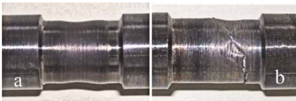
Figure 11. Shape of the cross-weld, all-weld-metal sample after the ACT terminated before entire fracturing (a), and of weld's HAZ with the crack following the HAZ's direction (b).
