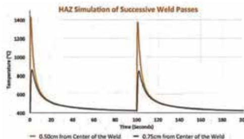
Figure 29. Thermal graph of two-cycle HAZ simulation on Gleeble [9].
