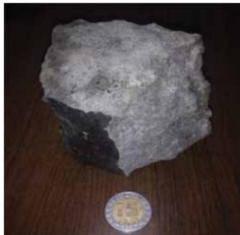
Figure 9. Basalt hand specimen collected at Station 5. The white surface has been exposed and chemically altered, while the fresh portion appears black.
