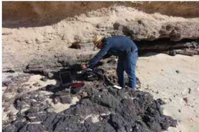
Figure 5. Measuring basalt with the spectrometer; the PC control and record measurements. At Station 2, two types of materials were sampled: Basalt and white tuff.
