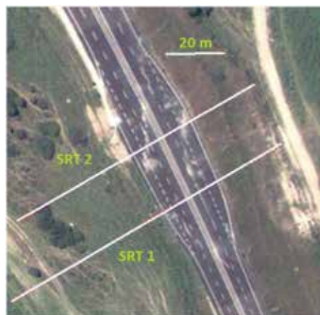
Figure 13. Position of the two seismic refraction tomographies.
