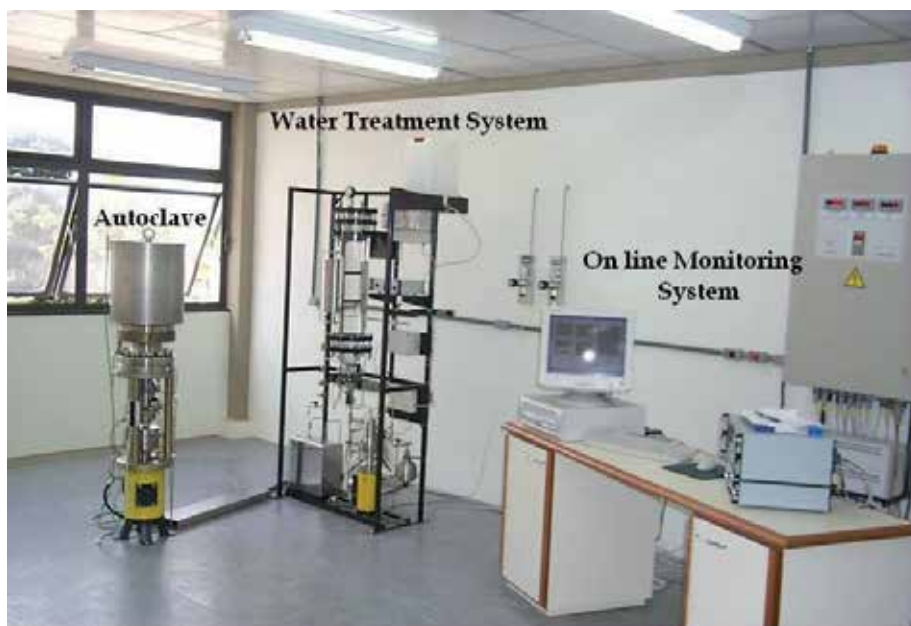
Fig. 8. Photo of the installation of SCC tests.
