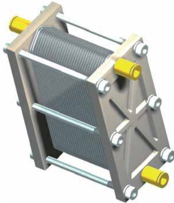
Fig. 2. Schematic design of an air-breathing PEMFC stack
