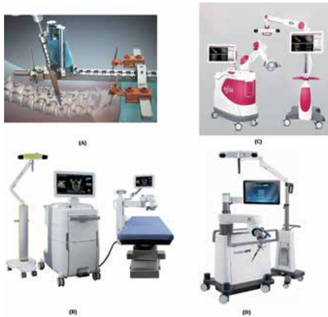
Figure 1. Systems for robotic-assisted spine surgery: Mazor Renaissance ® (A), Mazor X ™ (B), ROSA ® (C), and ExcelsiusGPS ® (D).
