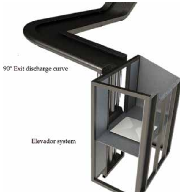
Figure 6. Workstation proposed redesign. It includes a system transport of 90° exit discharge curve and an elevation system.
