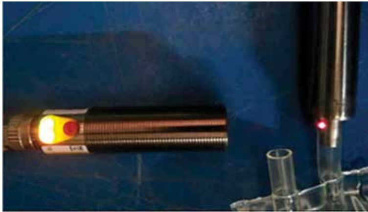
Figure 7. Photoelectric sensor in filling nozzle for automatic filling.
