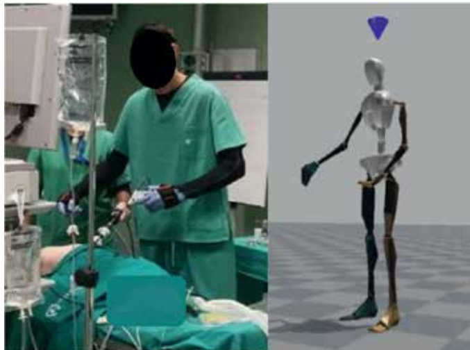
Figure 19. Sensorized surgeon with inertial measurement units (IMUs) and biomechanical model used by XSens.
