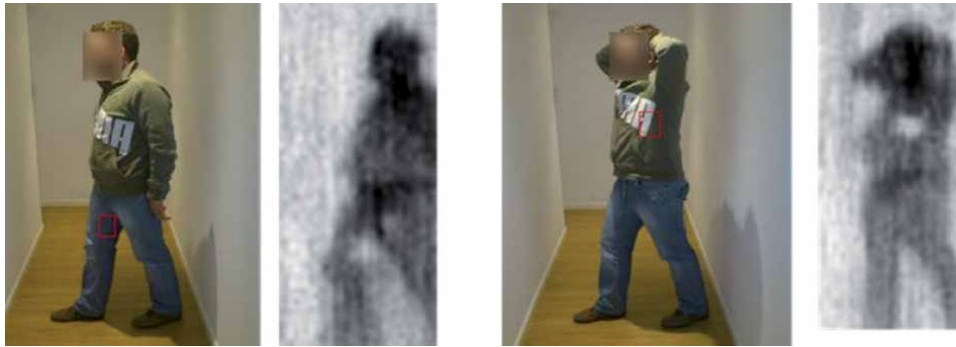
Figure 3. Automatic object and potential threat detection (ATD) on processed millimeter-wave image on the left and privacy protection output to operator on the right.
