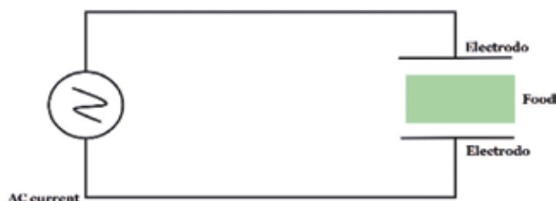
Figure 4. Schematic representation of the RF heating process. Source: Marra et al. [31].
