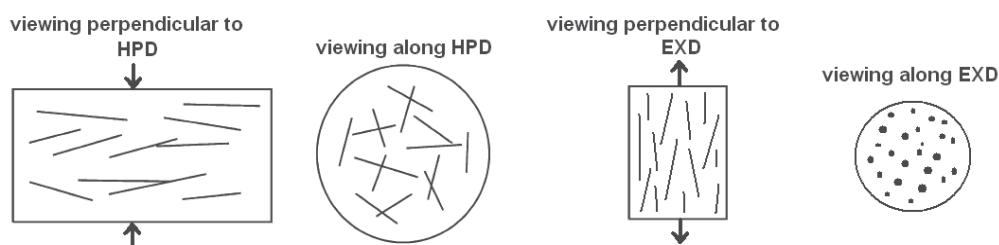
Fig. 6. Schematics showing the preferred orientations of \text{SiC} whiskers which result from the hot-pressing and extrusion-based processing methods. The processing directions (HPD and EXD, respectively) are marked by arrows. HP figures after Mebane and Gerhardt, 2006 (John Wiley & Sons).
