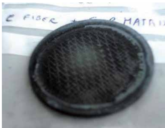
Fig. 5. Picture of the emitting surface of the sample CVDed \text{SiC} coated \text{C/SiC} after the emissivity experiment carried out at air pressure of 200 Pa increasing the temperature from 1000 K up to about 1900 K.
