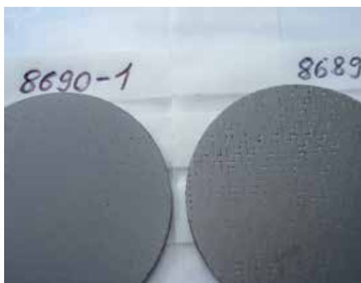
Fig. 9. Pictures of two CVDed SiC coated C/SiC specimens obtained by physical vapour infiltration.
