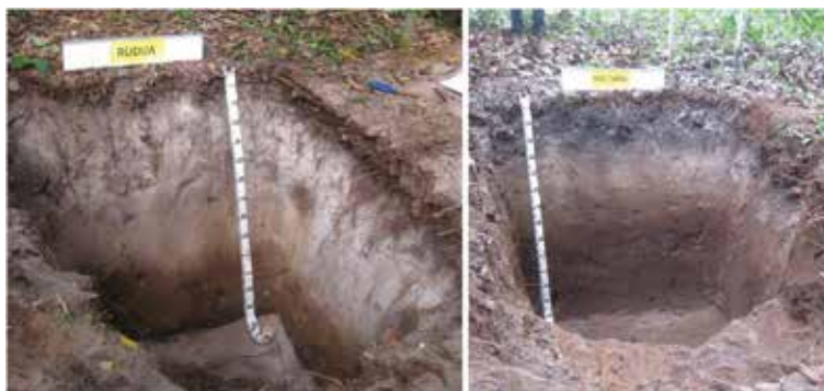
Figure 1. Examples of typical soil series (Rudua and Rhu Tapai soil series) under beach ridges interspersed with swales (BRIS) system in the East Coast of Peninsular Malaysia compose more than 90% of sand.
