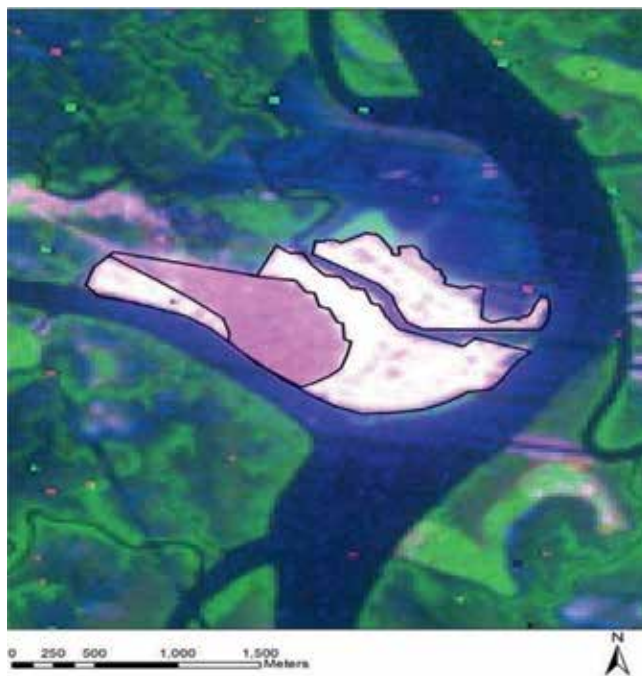
Figure 2. Dredged and sand filled areas in Buguma, Niger Delta, Nigeria. The white patch indicates the sand filled area while the green patches indicates mangrove forest that is still standing. The white patches sum up to give a total of 4.2 million m 2 of mangroves removed in 1984. This estimate was made using Arc GIS [9].
