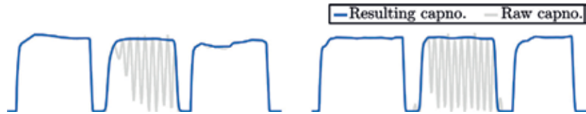
Figure 14. Examples of artifact suppression method performance. Original capnogram with clean and distorted respiration cycles is depicted by the solid gray line. Filtered capnogram (in blue) superimposed to the original capnogram.
