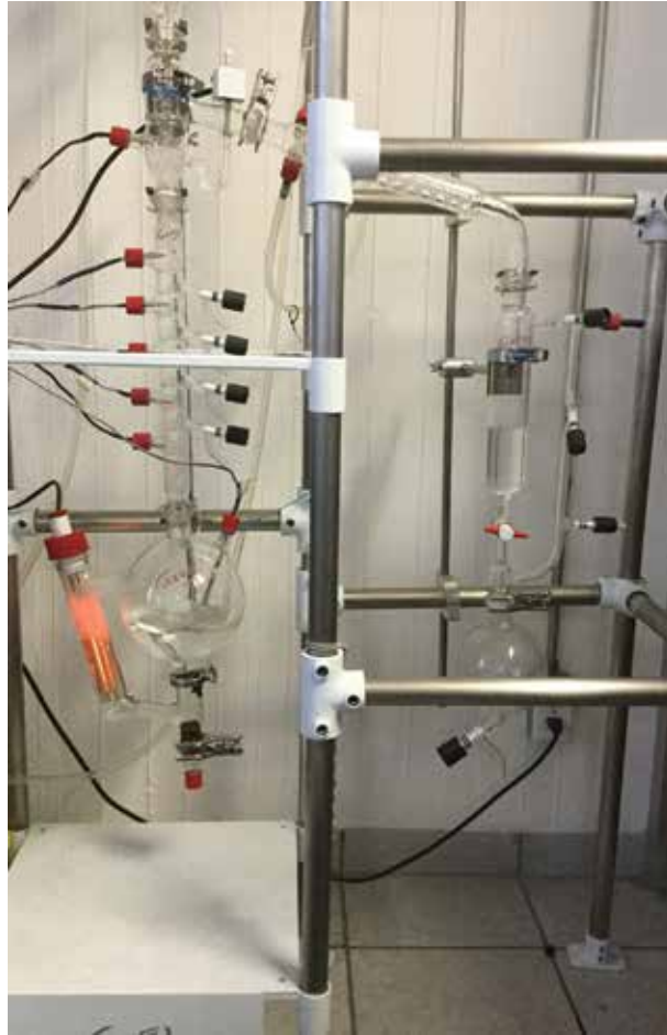
Figure 2. EDF-1000 distillation pilot plant.
