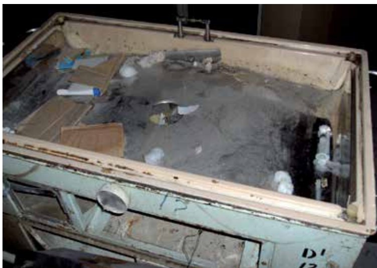
Fig. 2. An incubator carcass showing the inside immediately below mattress tray (removed); system was in use as is when retrieved
