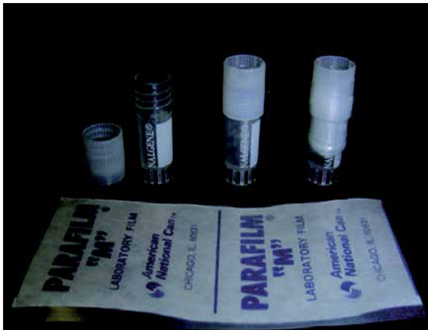
Fig. 3b. 2 ml Nalgene cryogenic vials (Thermo Fisher Scientific, Wiesbaden, Germany) (3b), filled with Ringer buffer and tightly sealed (e. g. with parafilm, American National Can GmbH, Gelsenkirchen, Germany).
