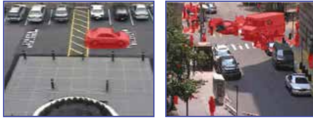
Fig. 2. Keyframes of example videos. (a) Sparse traffic scene; (b) Crowded activity scene. Red overlaid regions in the image represent the areas occupied by foreground moving objects.
