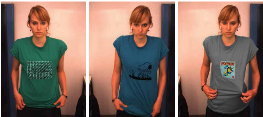
Fig. 9. Tracking and retexturing clothes in an augmented reality application (left: original frame with mesh)
