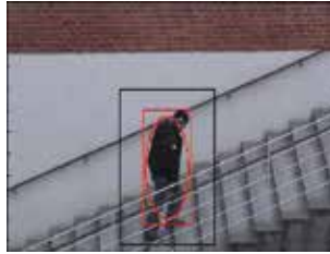
Fig. 2. Foreground and background regions. Red rectangle: a foreground object region; Black rectangle: the searching area. The area between the black and red rectangles is the background region. Red ellipse: maybe used for some objects (e.g humans) to minimize the possible inclusion of background points around the four corner areas.
