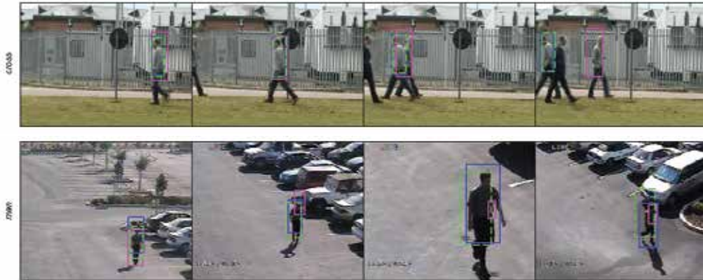
Fig. 5. Example video frames with output of the tracking algorithm output superimposed: DSSIM solid blue rectangle, SSIM-PF dashed green rectangle and MS solid magenta rectangle
