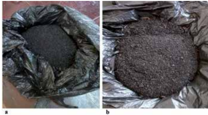
Figure 4. Biochar made from sawdust; a and b represent milled biochar and biochar in granular form respectively.
