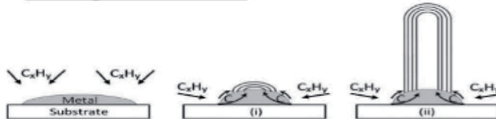
Figure 4. Schematic diagram of growth mechanisms of carbon nanotubes.
