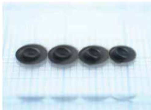
Figure 2. Tungsten nanoparticle deposits, obtained after four different deposition runs, collected on glass substrate.
