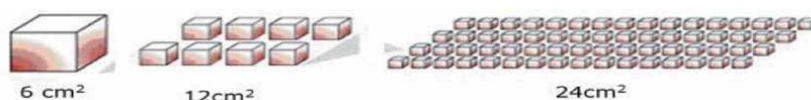
Figure 3. Novel properties of nanoparticles: surface area per unit weight increases, so more atoms come on the surface to interact occurred in nanoparticles.
