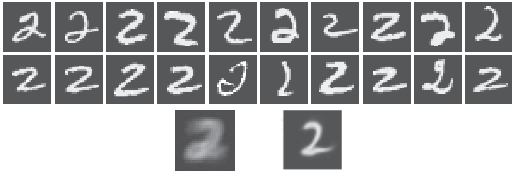
Fig. 5. Naive arithmetic mean (lower left image), mean image \hat{Z}_n (lower right image) based on 20 images of the digit "2" (upper rows).
