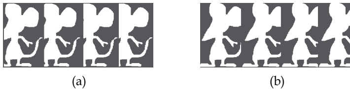
Fig. 10. Examples of occulted shapes from a model in MPEG-7 CE-Shape-1. (a) From left-occulted objects; they are occulted by 5%, 10%, 15% and 20%. (b) From right-occulted objects; they are occulted by 5%, 10%, 15% and 20%.
