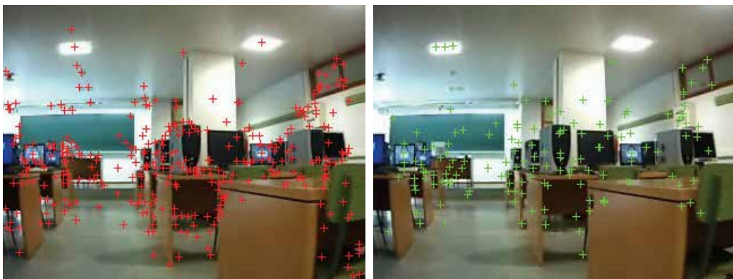
Fig. 3. SIFT (left) and SURF (right) keypoints computed for the same frame.
