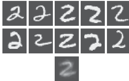
Fig. 3. Naive mean (two first rows) of a set of 10 images (Mnist database, 28 \times 28 pixels images, see LeCun et al. (1998) for more details on this data set) and naive arithmetic mean of these images.
