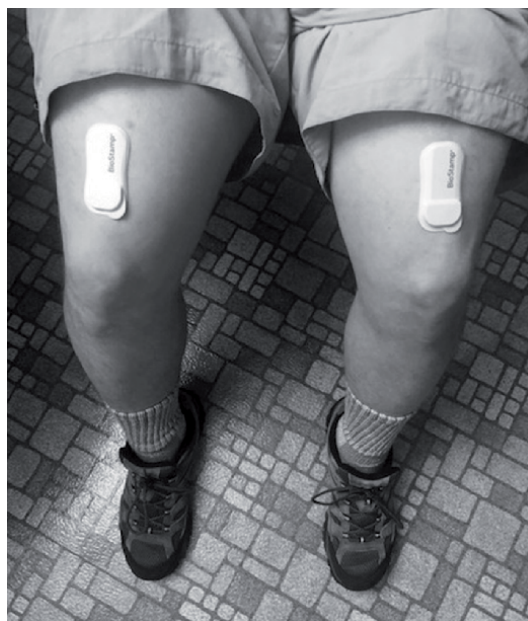
Figure 5. The BioStamp nPoint conformal wearable and wireless inertial sensor system mounted about the femur for the quantification of hemiplegic gait [91].
