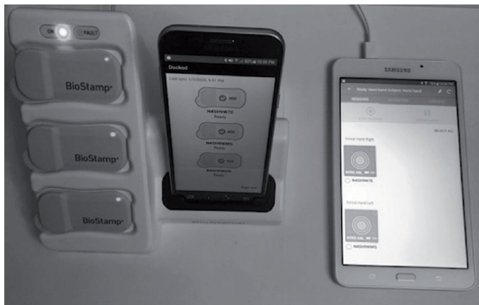
Figure 4. The BioStamp nPoint conformal wearable and wireless inertial sensor system and supporting devices, such as docking station, tablet, and smartphone [90].
