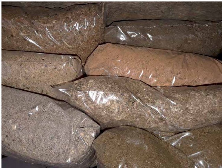
Figure 3. Remediation experiment using ground parts of mangrove ( Rhizophora spp. ) and Nypa palm ( N. fruticans ).
