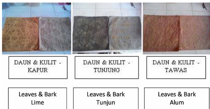
Figure 4. Batik fabric coloring from mangrove waste extraction with lime, tunjung and alum fixations.
