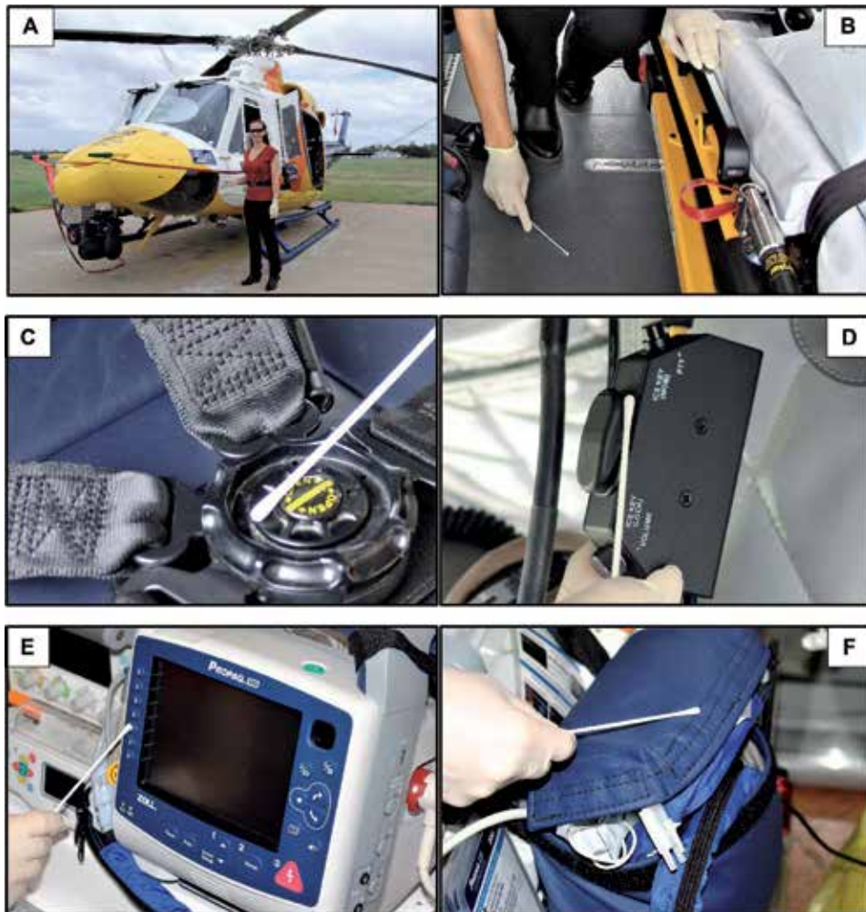
Figure 1. Sites for microbiological swab sampling for detection of bacterial contamination inside a helicopter air ambulance. Following discussions with paramedic staff and pilots five areas of the aircraft (A) were considered to have a high frequency of contact by emergency crew and patients. These locations were: (B) the floor surface between the emergency crew seats and patient stretcher; (C) the seat belt buckle on the emergency crew seats; (D) the hand piece of the Citizens' Band radio; (E) the buttons on the display panel of the cardiac monitor/defibrillator; and (F) the blood pressure cuff storage bag [13].
