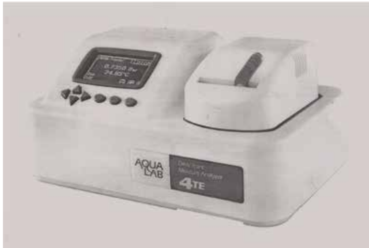
Figure 8. 4TE model AquaLab moisture content—water activity measuring instrument. Source: METER Group, Inc. [71].
