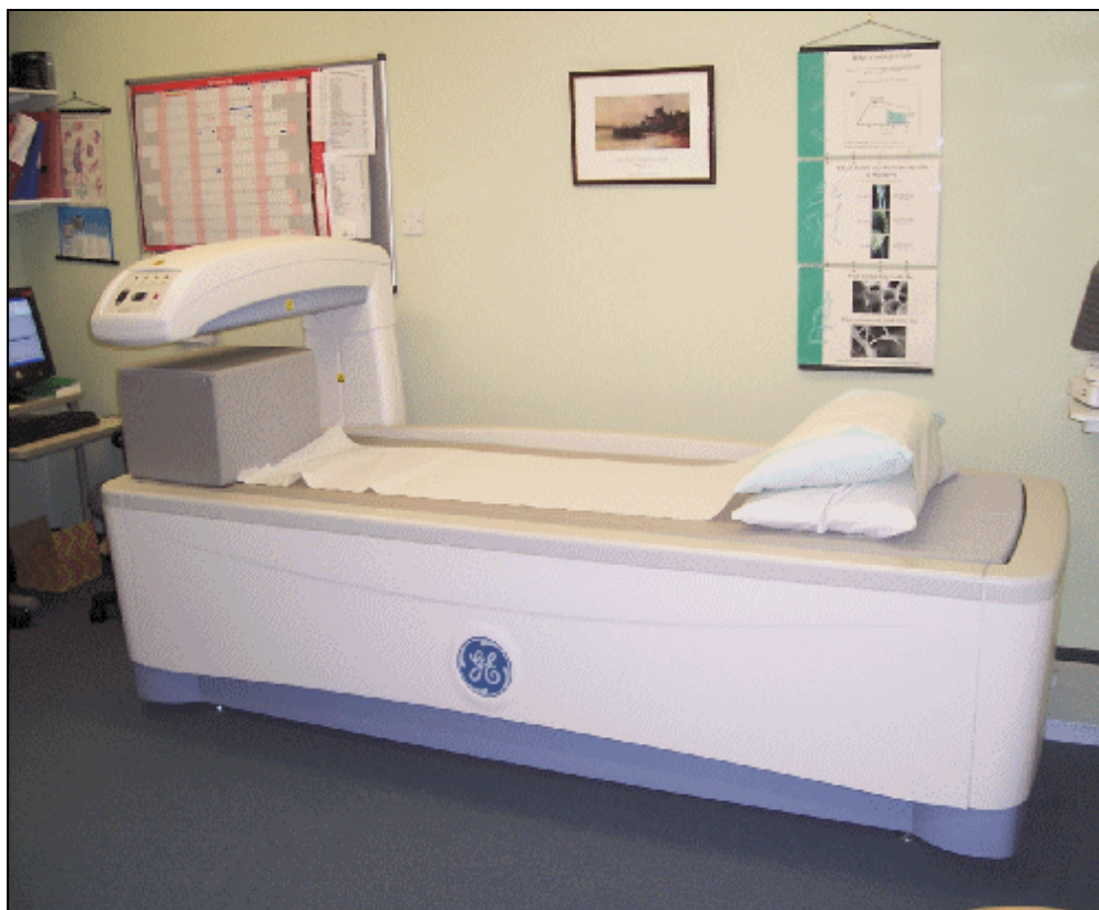
Fig. 4. A scanner used to measure bone density with Dual Energy X-ray absorptiometry.
