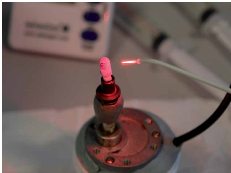
Figure 3. A zirconia dental implant placed in a rotational motor and treated with PDT 2 for 60 seconds.
