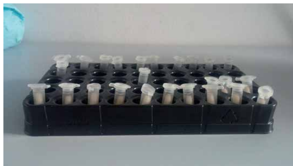
Figure 1. Implants placed in Eppendorf tubes containing bacterial suspension. Implants covered in their entire length by the bacterial suspension.
