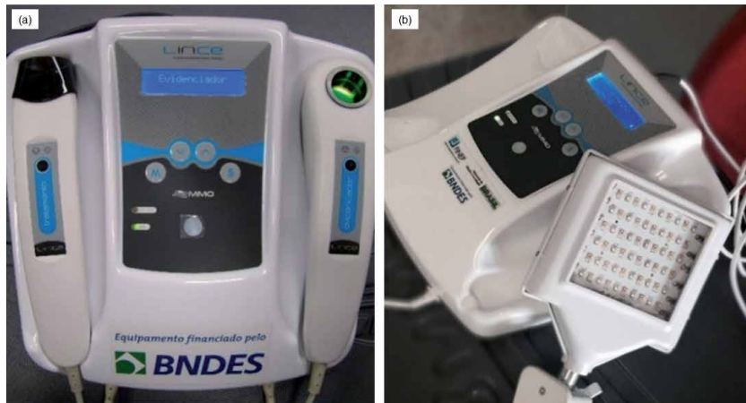
Figure 1. (a) LINCER® equipment (MMOptics – Brazil): left - treatment system emitting at 630 nm; right - diagnostic system emitting at 405 \pm 10 nm. (b) Square illumination of the LINCER® accessory emitting at 630 \pm 10 nm.
