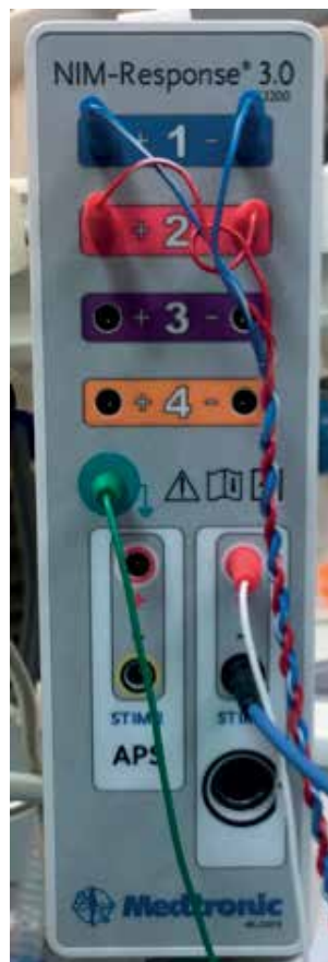
Figure 3. Stimulation and recording sides are combined on the interconnect box, through which they connect to the monitor.
