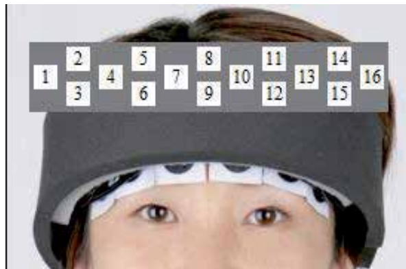
Fig. 3. Measuring points and headset. (Spectratech, Inc.)
